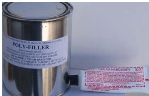
4a) The Poly-filler is prepared by adding 3% to 5% cream hardener to the filler. The mixed material has to be used within 5 minutes. Place three small, separate piles of the filler on a piece of cardboard (or substitute), and squeeze a separate pile of cream hardener alongside each. The cream hardener should be about 1/20<sup>th</sup> of the filler.
